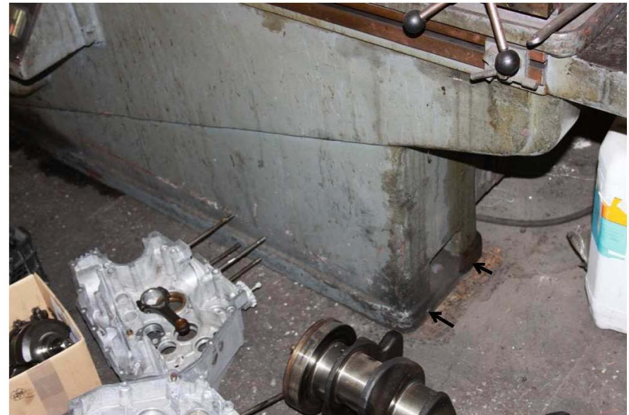
Sliding of heavy machinery towards North
