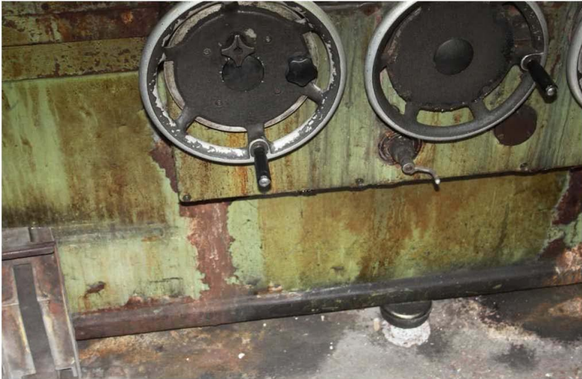
Sliding of heavy machinery with loss of the supports
