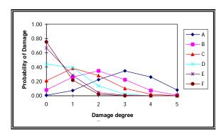
Figure 5: Probability damages matrix for intensity VIII
